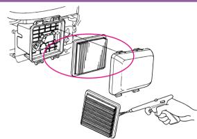
Wipe dirt from the inside of the air cleaner cover and air cleaner case, using a moist rag. Be careful to prevent dirt from entering the air duct that leads to the carburetor
