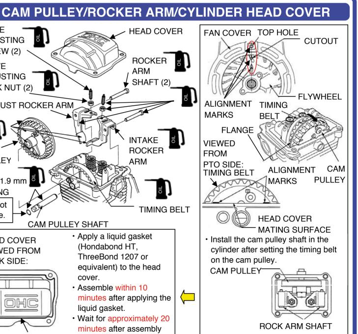
Install the rocker arm shaft from the
