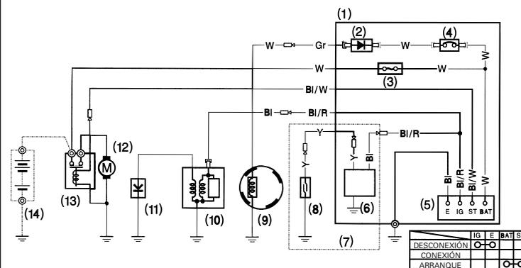
**Con alerta de aceite Oil Alert® y sin motor de arranque eléctrico**
