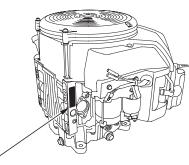
ENGINE SERIAL NUMBER & ENGINE TYPE LOCATION
