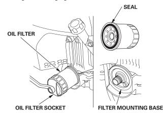
3. Clean the filter mounting base, and coat the seal of the new oil filter with clean engine oil.
