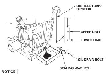
*Running the engine with a low oil level can cause engine damage. This type of damage is not covered by the* Distributor's Limited Warranty.
