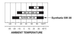
SAE 10W-30 or 5W-30 is recommended for general use. Use a full synthetic 5W-30 for starting/operating temperatures between 5°F (-15°C) and -13°F (-25°C). Other viscosities shown in the chart may be used when the average temperature in your area is within the indicated range.
