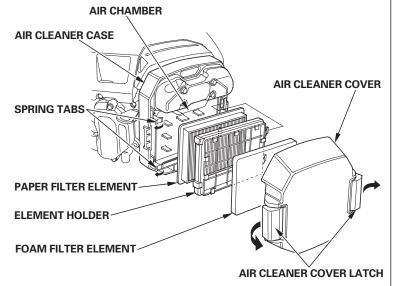
4. Inspect both filter elements, and replace them if they are damaged. Always replace the paper filter element at the scheduled interval (see page 6).
